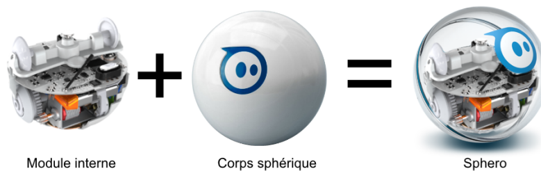
Figure 1 Constitution du Sphero
